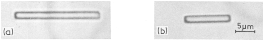
Figure 3 Optical micrograph of a disappearing needle-shaped void at 800°C: (a) 0 h; (b) 8 h.
